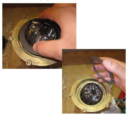
Step 5 Gently (so the output wires do not damage the driver) lay the sphere on the side of the casting.
