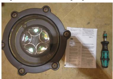
Step 3 Remove 2 screws from the inner ring that secures the sphere in place. **NOTE:** Place the glass on top of a sheet of plastic to avoid scratching.
